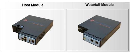
Modules are individual units that can be arranged together in a variety of hardware configurations within a single WF-500 cabinet.
